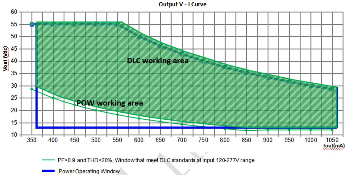
Note: When the output current is set, the output voltage is automatically limited within the curves.
