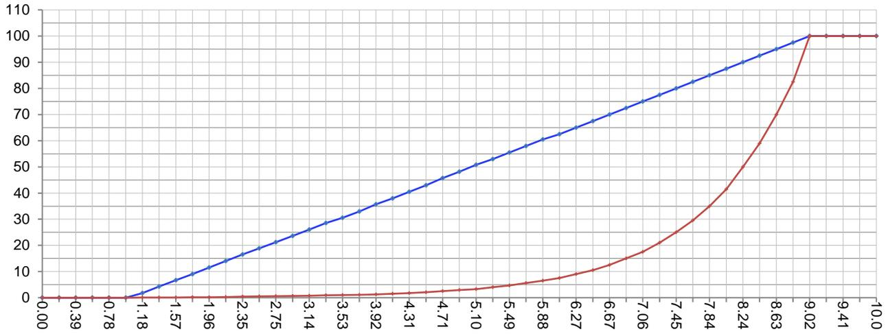
**0-10V Dimming Curve @ Minimum dimming set to 10% and dim to off :**
