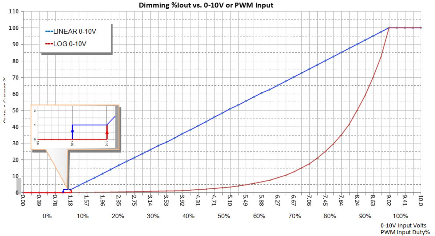
0-10V Dimming Curve @ Minimum dimming set to 10% and dim to off :
